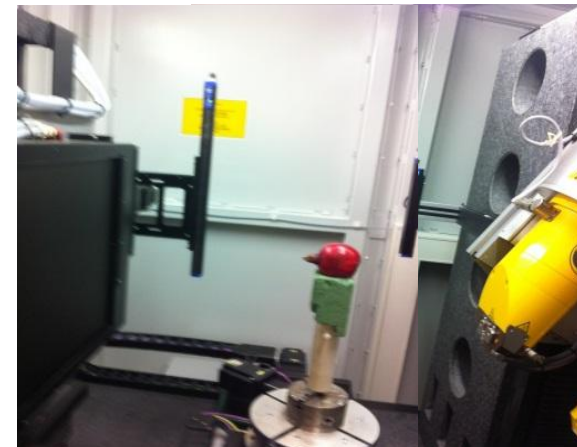
Microfocused X-ray computed tomography for non destructive detection of false codling moth in pomegranate fruit.
